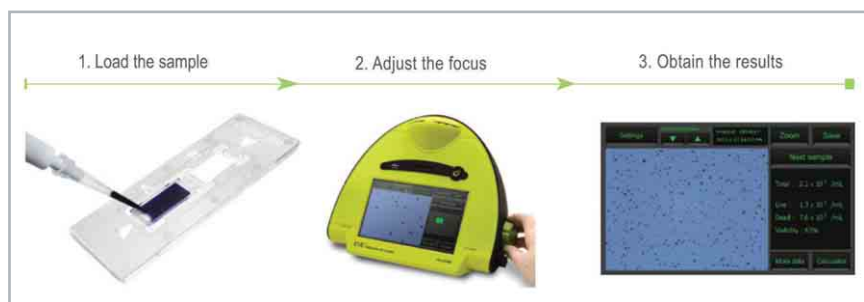
Figure 1. Automatic cell counter, EVE™ Uses a disposable chamber that contains two enclosed chambers can count the cells with just 3 steps. Step 1. Load the sample, step 2, adjust focus, step 3. Obtain the results.
